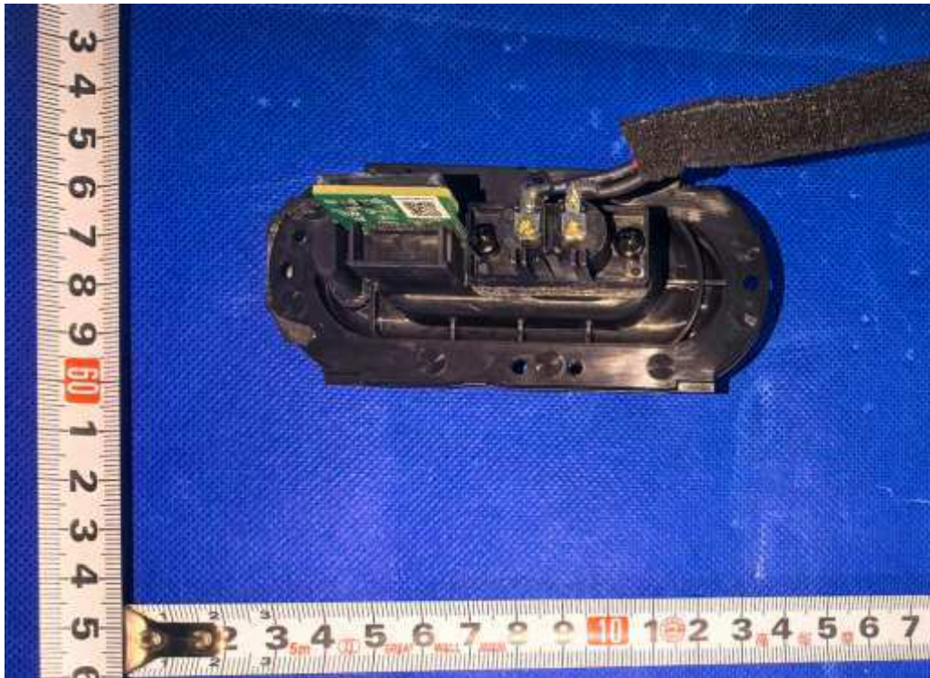
Figure 31: Internal view for appliance inlet and USB-C board
